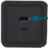
The **Type-A** USB connector is a standard USB port, used for standard cable connection interface for personal computers and consumer electronics devices.
