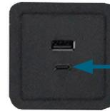
The **Type-C** USB connector is a smaller USB port.
