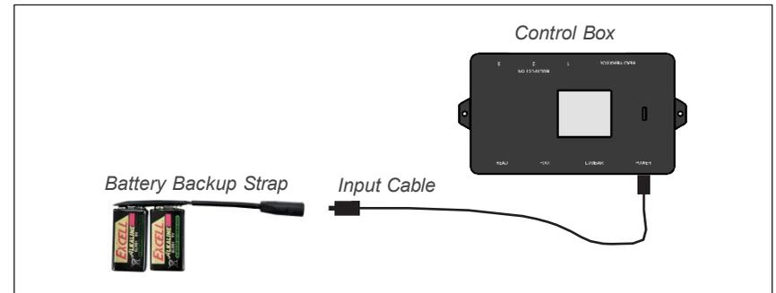
**Note:** Detach the Battery Backup Strap after the emergency is over, as the system will continue to draw power from the batteries even if not in use.
