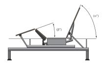
section for various configurations of the mattress support platform shall be  $\pm$  3°, which translates to a tolerance of up to  $\frac{3}{2}$ ".
